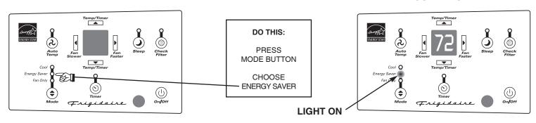
**Note:** In this mode, the fan will continue to run for another 3 minutes after the compressor shuts off. The fan then cycles on for 2 minutes at 10 minute intervals until the room temperature is above the set temperature, at which time the cooling system turns back on.
